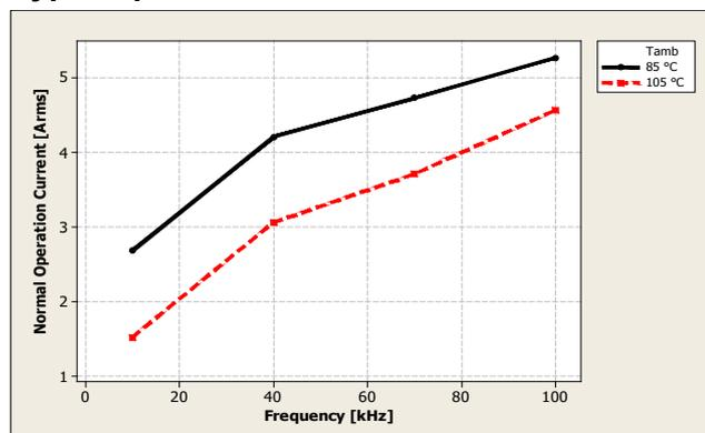
Measurement performed at  $V_{op}$ .
